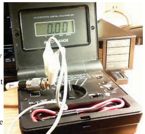
Figure 3. Simple go/no-go continuity test for cable/connector.
