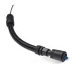
This component is commonly employed on Cell Towers for a connection to Remote Radio Units. The IP-67 rated gland is water and dust ingress protected, corrosion resistant and designed with a bayonet-style locking system for secure and easy mating. The protection sleeve protects the last foot of the connection to an RRU.
