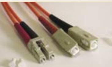
Fiber optic cable is also highly resistant to electromagnetic noise produced by radios, motors or other nearby cables. The two most common types of fiber cables are multimode and single mode. The more expensive multimode will handle several thousand modes of signal transmission over medium distances, while single mode provides an optimized transmission of a single carrier over a great distance. Common connectors for fiber are ST, SC and LC.
